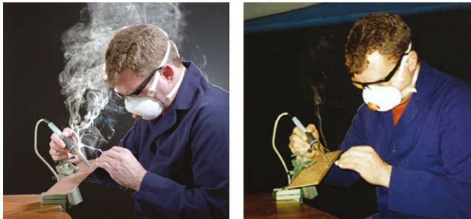
Figure 45 Soldering with and without Tyndall illumination
