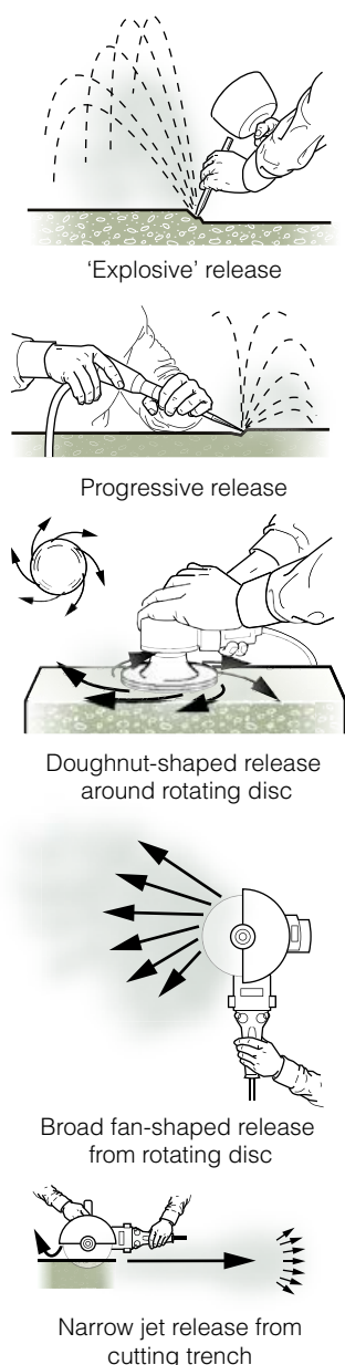
Figure 5 Processes and sources in stonemasonry
